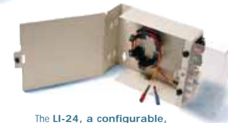
The LI-24, a configurable, wall-mounted, optical fiber interconnect unit , accepts up to four 6-Pak plates. Each LI-24 is outfitted with internal fiber management rings and cable ties.
