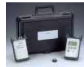
The FLT4 Optical Loss Test Set is an easy-to-use and inexpensive solution for attenuation testing of multimode systems. The test set consists of a dual wavelength optical power source and optical power meter in a rugged plastic case, complete with ST adapter cap and operation manual.
